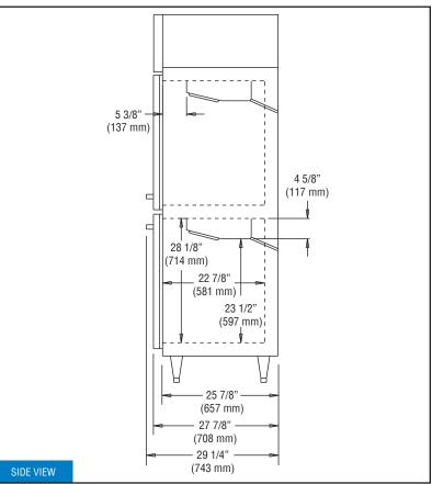
**IMPORTANT NOTE**: If the cabinet is located directly against a wall and/or under a low ceiling, a minimum clearance of 12" is required on top and 3" on sides and rear.
